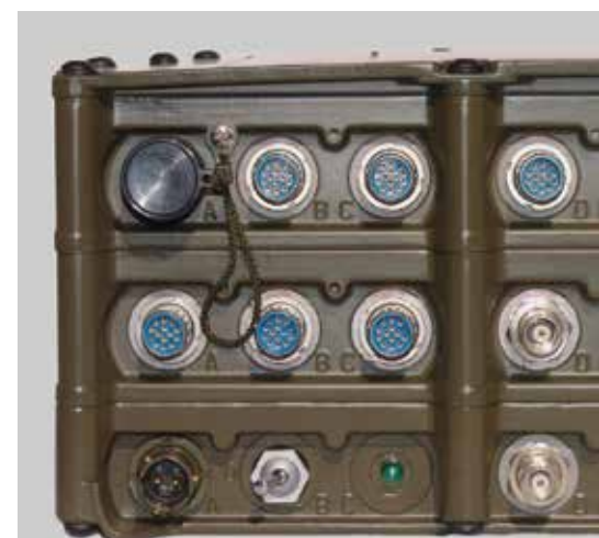
CMSU-IP (Central Multimedia Switching Unit)
